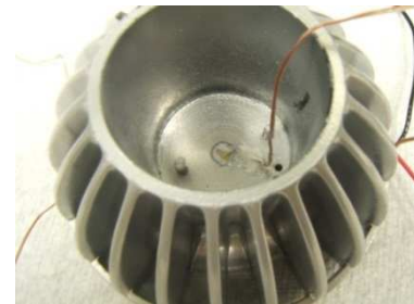
Thermocouple attached to back plate
