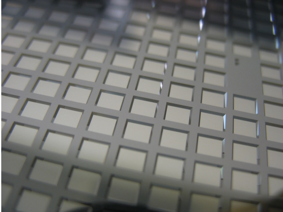
Si/glass cap wafer with tapered reflector edges
