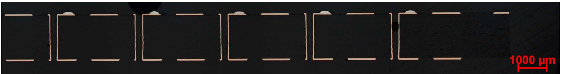
Crosssection of PCB with solder depot
